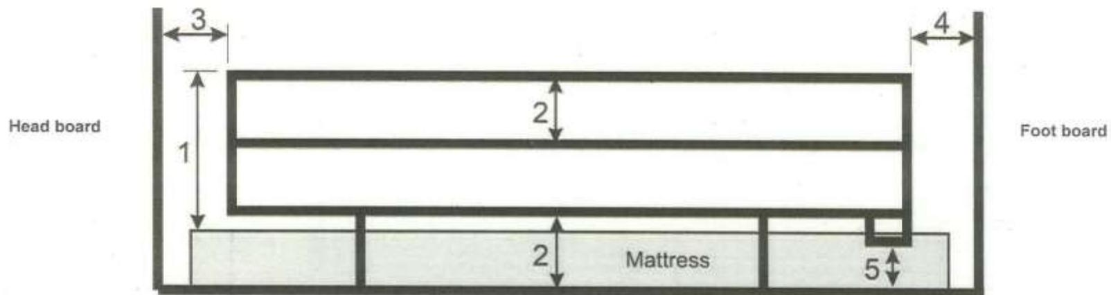
Diagram of side view of bed with cantilever side rails
